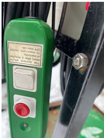
Figure 23 Voice Control - Toggle switch Mutes and Activates Voice. Red button is a manual Trigger.
