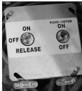
Figure 17 Hydraulic and Trap On/Release Switched - Release Bird and turn off pump when done.
