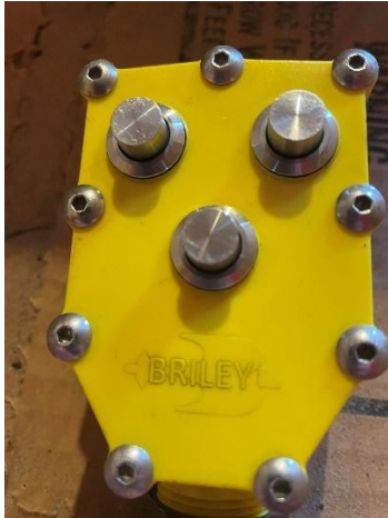
Figure 12 Push Button Handheld - Left - High Bird, Right - Low Bird, Bottom - True Pair
